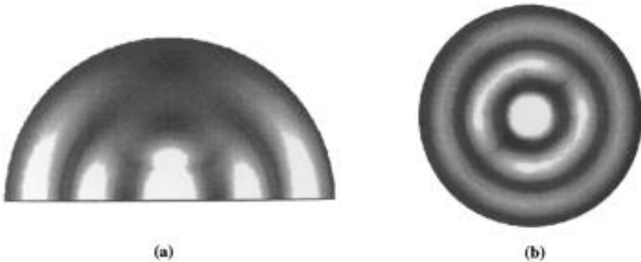
FIG. 15. Computed (a) electric (b) magnetic field magnitude in the vicinity of \lambda/12 dipole.
