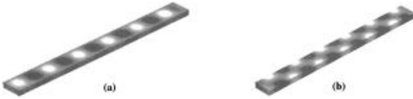
FIG. 12. z -component of (a) electric field (b) magnetic field in PML terminated waveguide.
