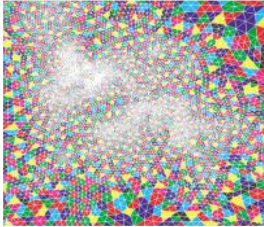
FIG. 15. Agglomerated elements: Rectangular domain with unstructured triangular elements.
